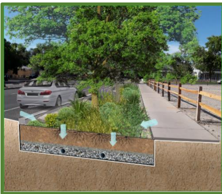
This illustration shows a cross section of what the bioswale looks like once planted and the trees and plants have grown in.
